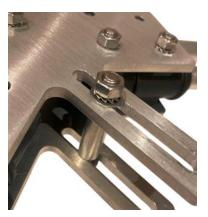
**Step 8 (2m version only):** Insert the remaining M6 bolts, followed by a shakeproof washer, through the plate holes. Secure them with another shakeproof washer and an M6 nut on the opposite side. Fully tighten these bolts, as they function as a hairpin for impedance matching.
