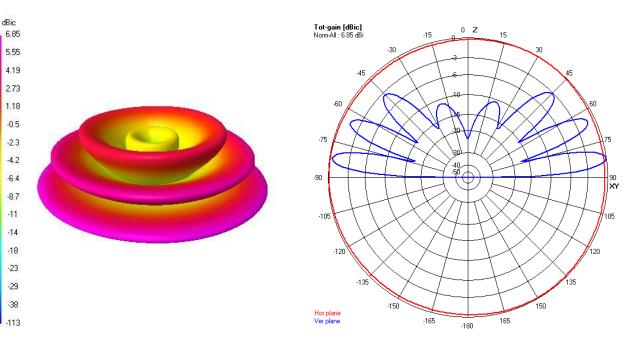
Fig 4. (70 MHz) 10m above ground - Antenna mounted on a 2" pole, 10m above ground.
