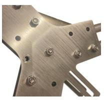
**Step 7:** Locate the tubular spacer and insert it between the two slot cuts protruding from the plates. This is the tuning stub, also referred to as the hairpin match. Insert an M6 bolt, followed by a flat washer (Ref I), through the hairpin match and the tubular spacer. Secure with another flat washer, a shakeproof washer, and an M6 nut. Only loosely tighten, as this will require adjustment for tuning later.
