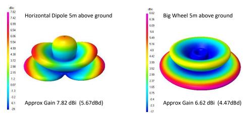
As evident from the models, the Big Wheel antenna still demonstrates negative gain compared to a dipole. However, as the 3D radiation pattern illustrates, the horizontal dipole radiates in only two directions (e.g., east and west), leaving no coverage in the north and south. In contrast, the Big Wheel antenna spreads its RF energy uniformly in all directions, making it one of the best horizontal omnidirectional antennas available.
