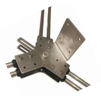
**Step 6:** Flip the antenna again and fully tighten all the M6 bolts. Add a shakeproof washer to the center bolts, followed by an M6 nut, and tighten securely. At this point, all nuts should be fully tightened.
